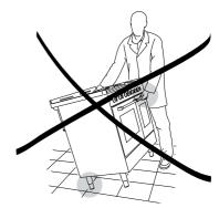
Figure 8 Incorrectly raising the cooker
